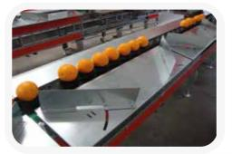
SYSTEM OF EXITS AND DISCHARGE The fruit is discharged from the trolley through computer-controlled solenoids. They tilt the trolley and release the fruit directly on the collection tanks.
